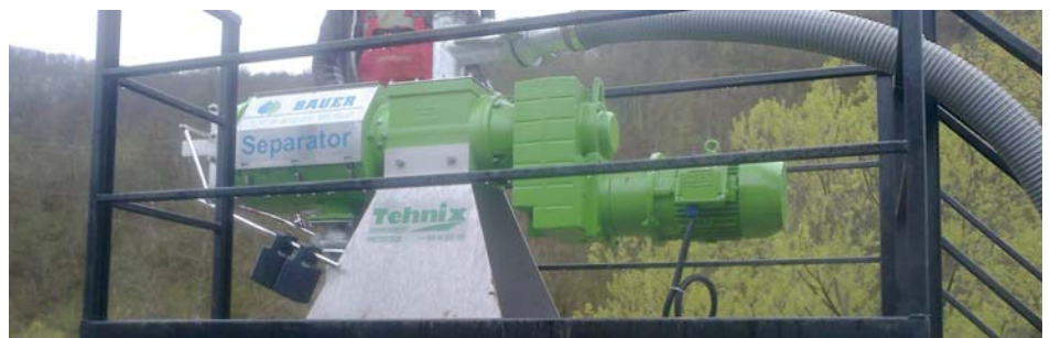
SLUDGE SEPARATOR FOR BIOREACTORS AND FARMS
