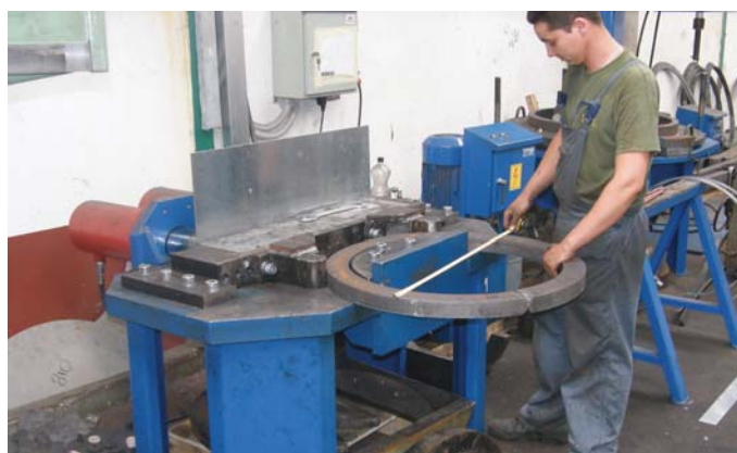
Flanges production by bending on special machine
