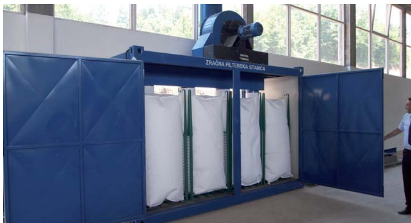
Air filter station - type 1 (2250 x 1650 x 2500), type 2 (4400 x 1650 x 2500)
