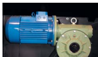
Drive worm unit for press-containers
