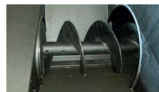
Driving worm, high pressing efficiency (1:10)
