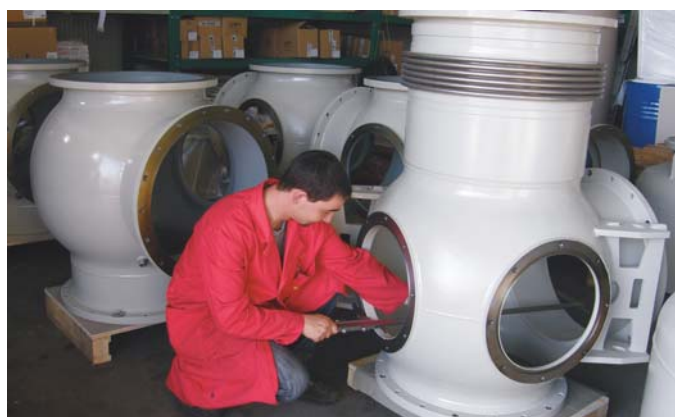
Final control of finished casings after painting
