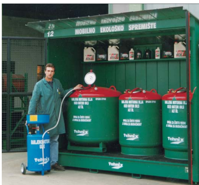
Collection of used motor oil in eco container
