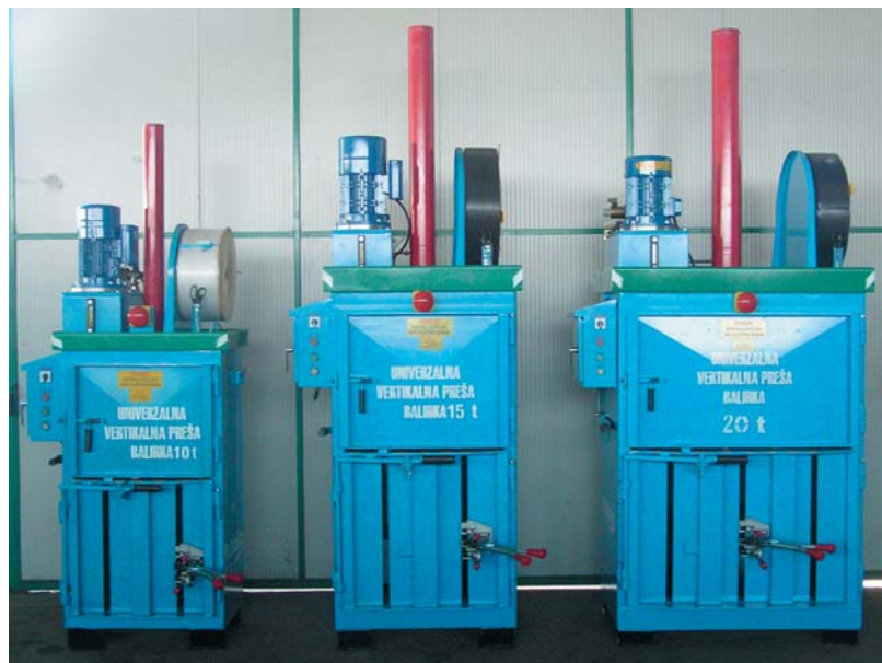
Baling press - vertical/pressure 10, 15 and 20 t
