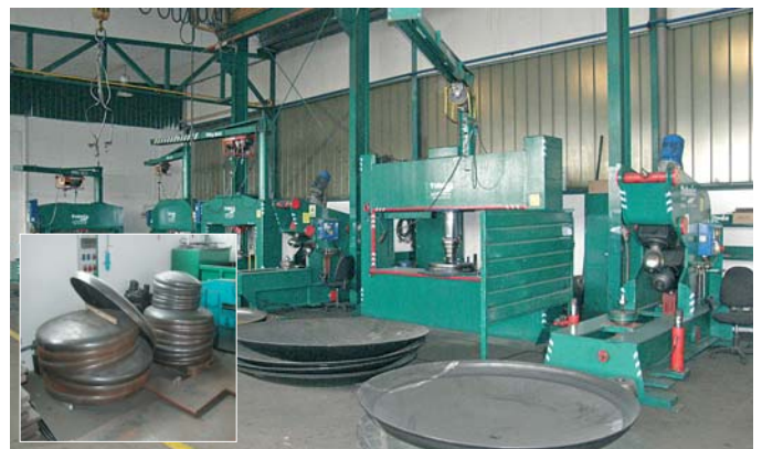
Technological line Tehnix for the production of floor steel plates 15 mm thick with a diameter of 500 to 3,000 mm
