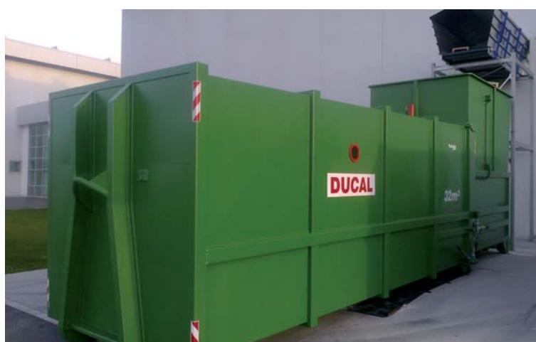
Special desing of two-part press-container with lifter
