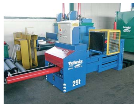
HPB-25 special version, pressure 10 kg/cm 2
